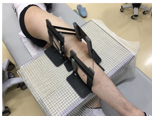
Figure 1. Knee Clamping Device. A knee immobilization device was fabricated to hold the knee joint in the extended position. In order to avoid inhibiting the mobility of the deep fascia due to the compression of the lateral part of the lower limb on the test side, one control plate was placed in front of the knee joint, and two control plates were placed distal to the thigh and proximal to the lower leg to immobilize the lower limb.
